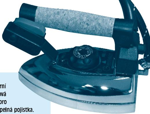
Electric steam iron model "U" with 4 m electric cable, plug and 3,3 m steam hose. Equipped with cork handle comfortable for handling and with high isolating performance, sole plate element and safety thermal fuse. Voltage 230 V/1ph, 50–60 Hz. Power 800 W.
